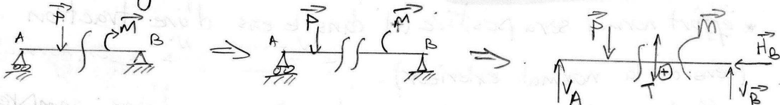
\*  $\sum F_x = 0 \dots\dots M(x) = 0$     \*  $\sum F_y = 0 \dots\dots T(x) = 0$     \*  $\sum F_z = 0 \dots\dots M(x) = 0$
